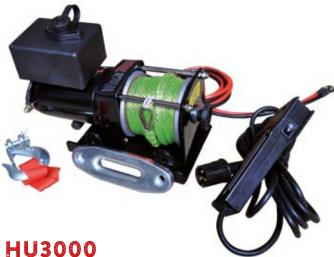
3,000lb (1,360kg) 1.34hp 12V DC motor, genuine Dyneema® SK75 rope 4.8mm x 12m, includes hawse fairlead, wired remote control, G70 1/4" clevis hook & mounting bracket
